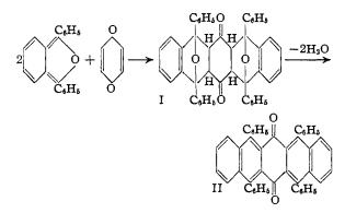
This new synthesis makes it possible to obtain symmetrical or unsymmetrical polyarylated pentacenes, which are only difficultly or not at all accessible in other ways. It also confirms the structure previously<sup>6</sup> assigned to II, which had been arrived at by an examination of the products of degradation. It is limited only by the nature
